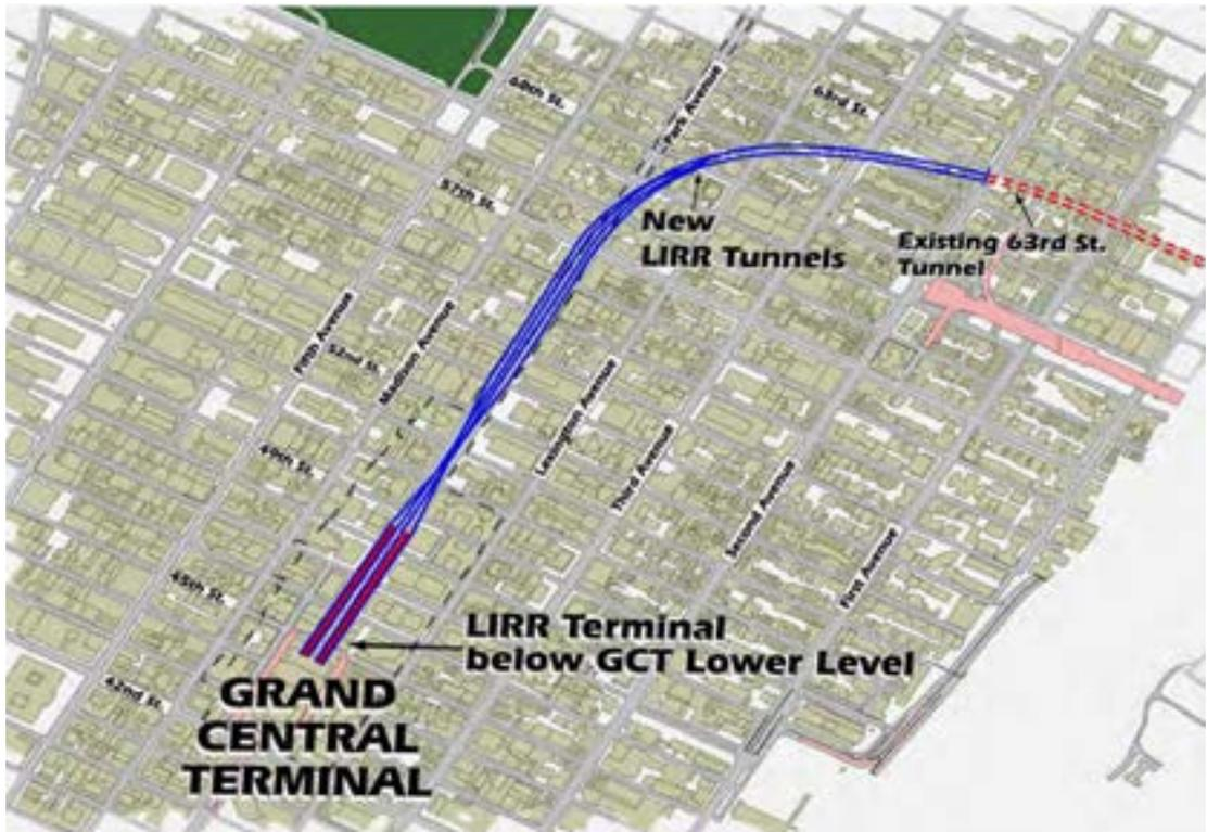
Access tunnels connect from railroad level of 63rd Street Tunnel under East River, completed in 1973
