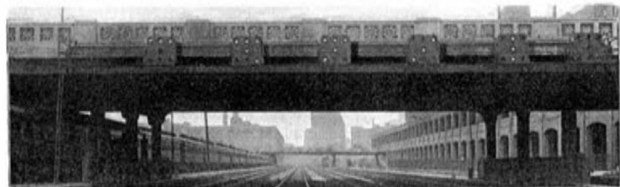
A View of the South Approach Tracks Showing Position Light Signals Mounted on the Facia of the Taylor Street Viaduct Pennsylvania Freighthouse in the Right Background
