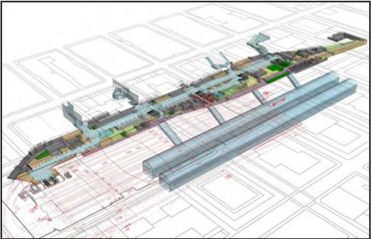
*Isometric drawing of proposed new ESA station concourse and tunnels under Grand Central Terminal, highlighting four connecting escalator banks*
